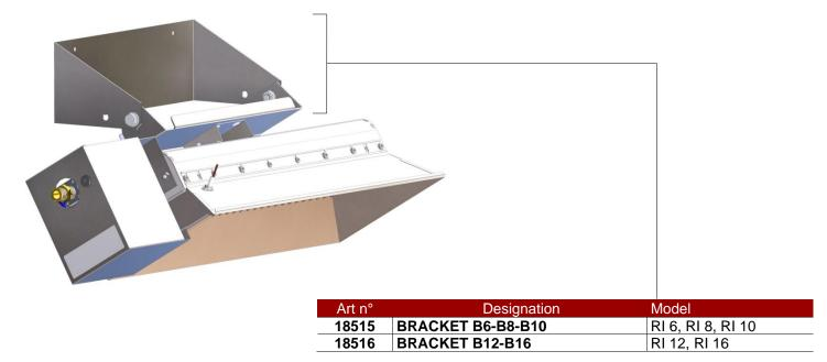
With these brackets, it is possible to use an 60 cm extension to deport the radiant from the wall.
