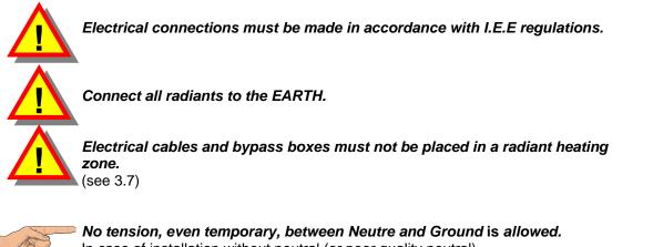
No tension, even temporary, between Neutre and Ground is allowed. In case of installation without neutral (or poor quality neutral), provide an insulation transformer to create an artificial neutral. To do this, connect a terminal of the secondary of the transformer directly to the ground.  $230V \sim I$ L + N + G To Control module
