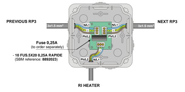
□ Internal electrical diagram of the heater
