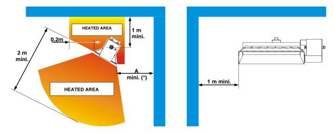
(\*) For an inclination "I" or a slope "P" between 20° and 35°, A=0.6m.
