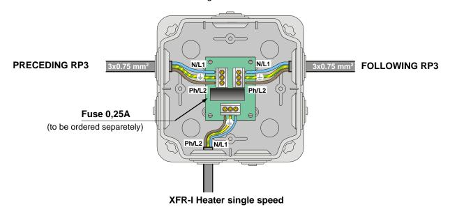
■ Wire RP32's as shown in the diagram below :
