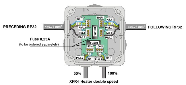
☐ Internal electrical diagram of the heater (by speed)
