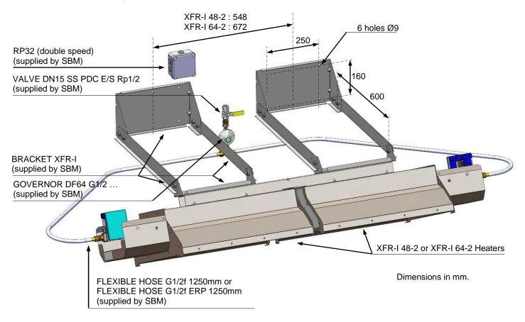
☐ Hanging example with chains or cables for XFR-I 48-2 and XFR-I 64-2
