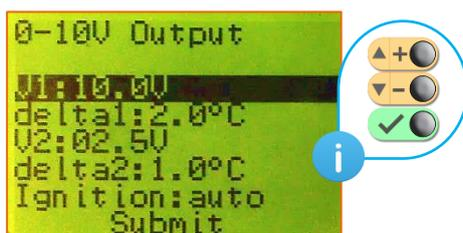
**V1** : the voltage corresponding to a temperature measured equal to :  $Setpoint - Delta1$ .
