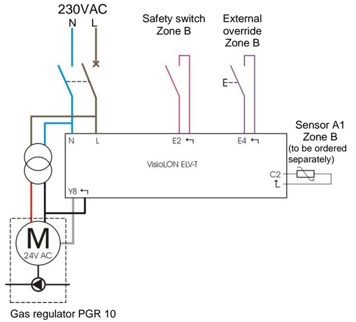
**2.5 Wiring of power supply**
