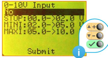
**STOP** : define the values mini and maxi of the 0-10V signal where the heating system will be off.
