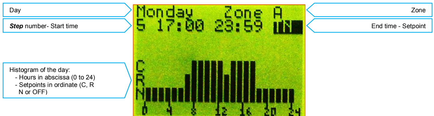
Choose the setpoint desired [TC : Comfort / TR : Reduced / TN : Night / OFF] (after validation, the screen go to the next step )
