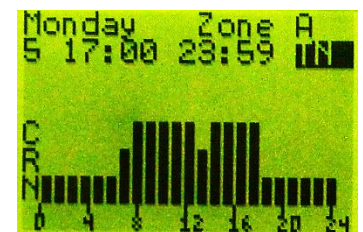
Choose the setpoint desired [TC : Comfort / TR : Reduced / TN : Night / OFF] (after validation, the screen go to the next step )
